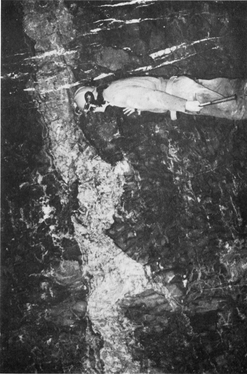
Plate 8. Irregular stratiform sulphide layer in 2-3 Lens showing thickening and depression near minor vein mineralization in foot-wall.
