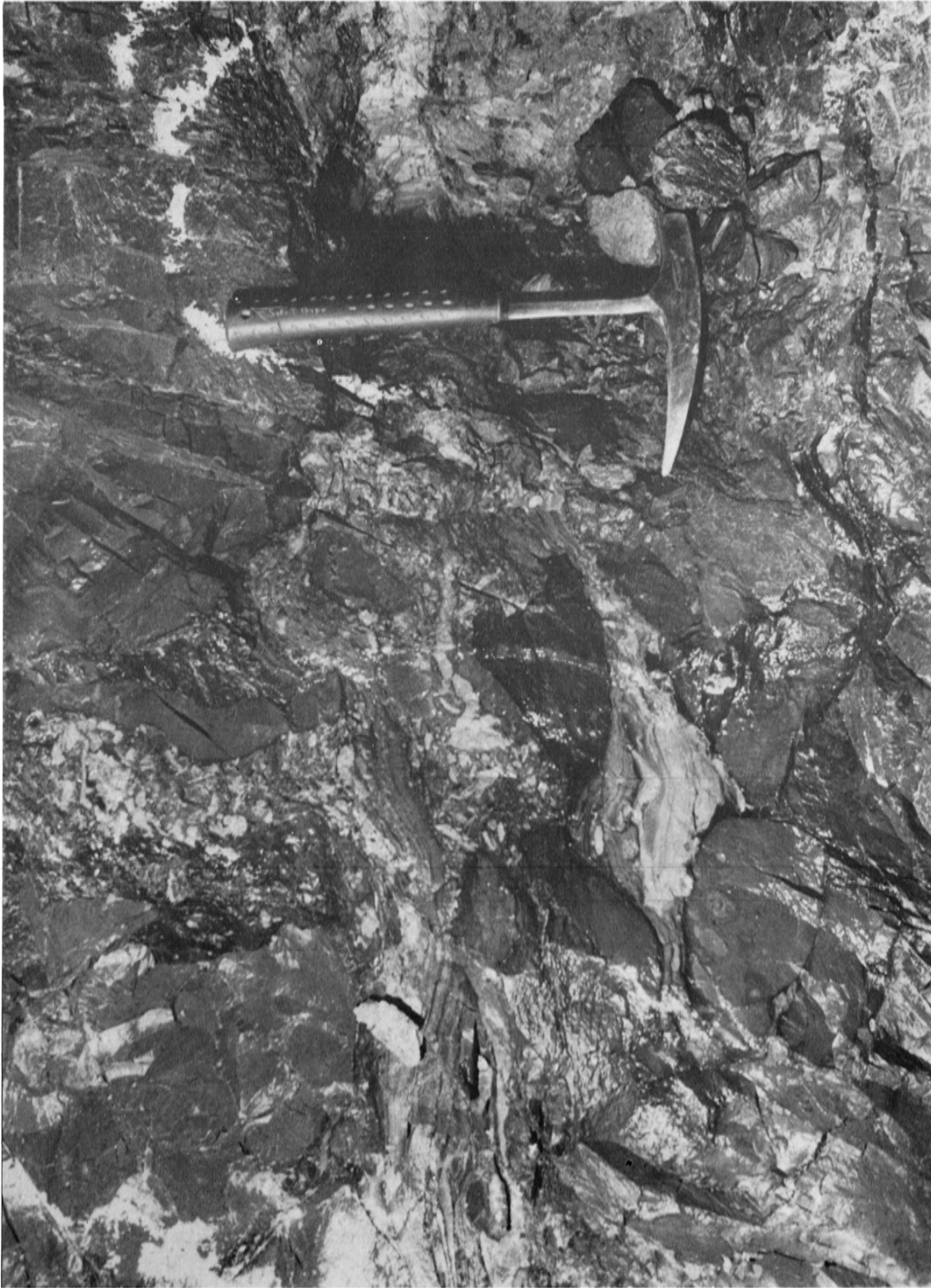
Plate 14. Complex mineralized breccia in 1-5 Lens. Irregular micrite clasts containing oncholites are enclosed by a mineralized matrix, containing dark argillite, laminated and layered sphalerite and minor galena. The micrites are undolomitized. (Hammer for scale).
