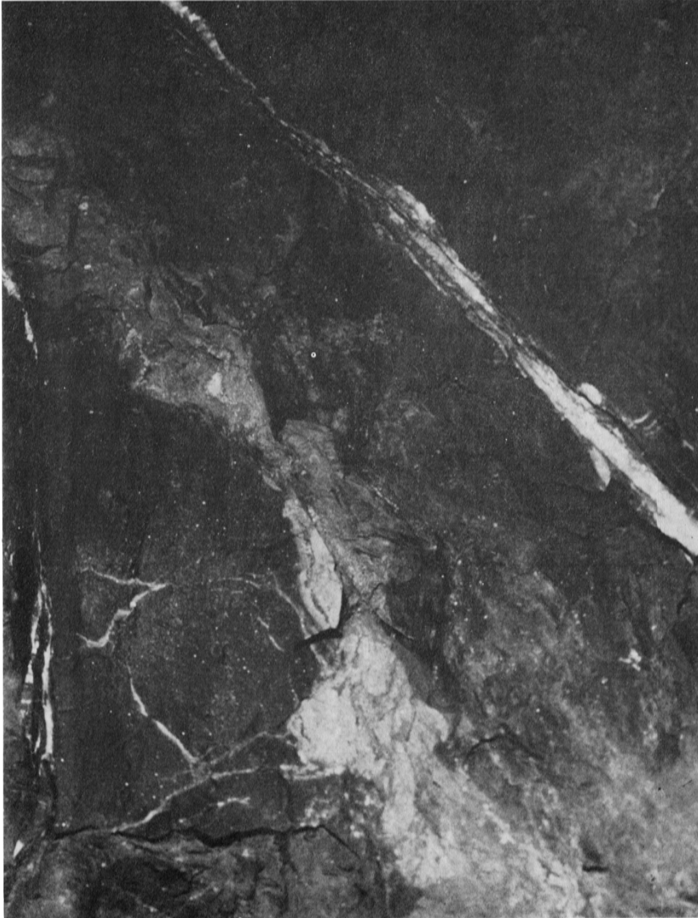
Plate 6. Irregular cross-cutting sphalerite vein cutting Muddy Limestone and followed by later shearing and carbonate veining. 10m below base of 1-5 Lens. (Width of frame 0.8m)
